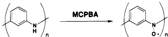
Figure 6. Conversion of poly( m -aniline) into poly( m -phenylene nitroxide).
